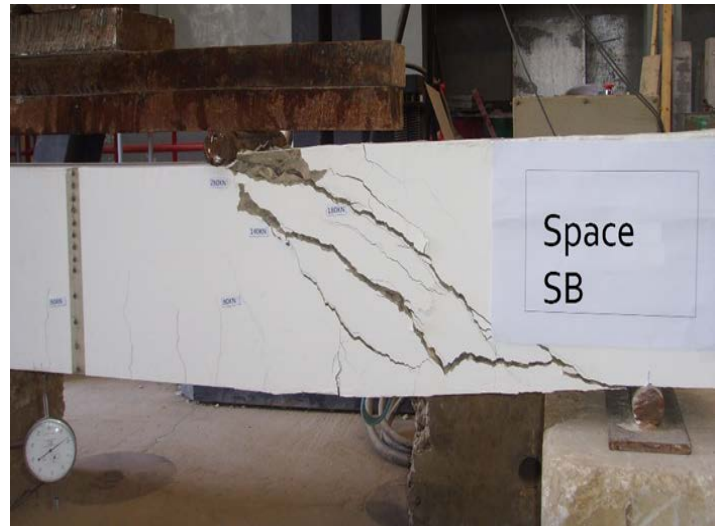
Fig. 7: Typical shear failure.
